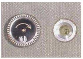
When the camera is loaded with 35mm film, you need to rotate the frame counter reset knob behind the frame counter ½ turn after every  $10^{th}$  picture. Rotating the reset knob causes the frame counter to return to 1. Otherwise, the counter will go to frame 11, 12 and then red dots with no frame spacing control. In other words, you will not get all of the pictures on your roll of 35mm film, the film will wind all of the way to the end without stopping. The
